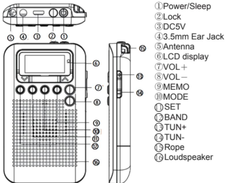
①POWER/SLEEP:For turning on and off the radio.adjust automatic shutdown.
