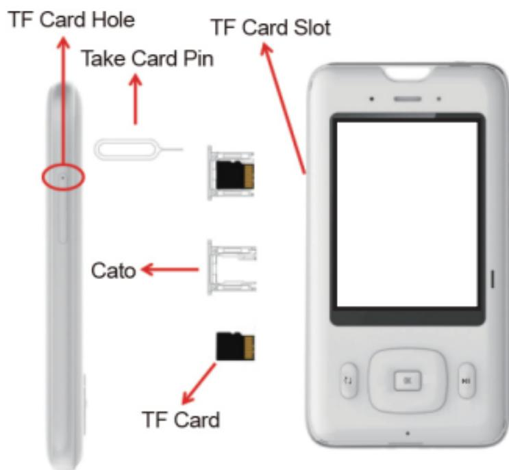
**Insert Card:** Put the TF card to the cato, then insert the cato into the card slot of the device (Please be careful not to reverse the direction of the card)
