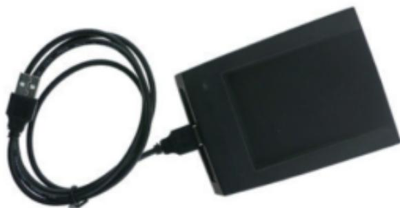
You need to install the driver for the first use of the tag writer (The drivers for Win7 and Win10). After the driver is installed, please check if the installation is successful or not as follows: My Computer--Management--Computer Management--Ports, if you could find the CP210X USB to UART, that shows done. (Figure 1)
